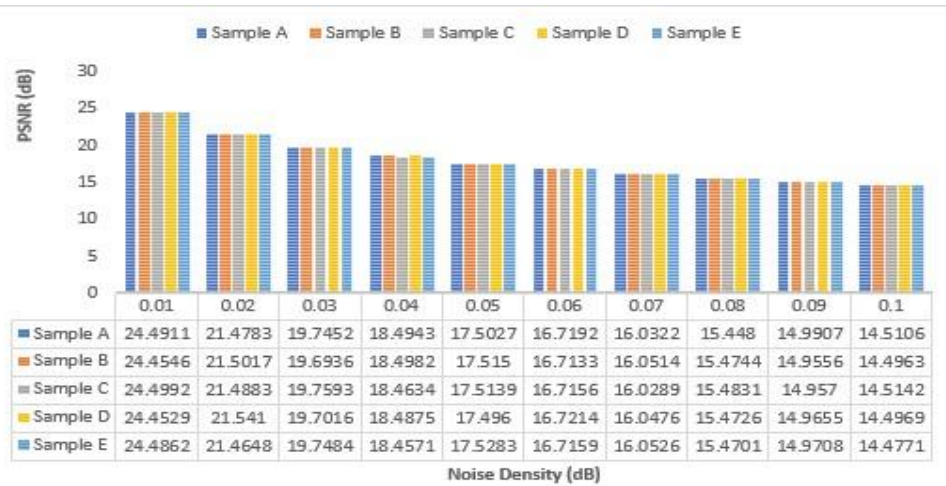
Fig. 6. PSNR (dB) value versus Noise Density for Sample A, B, C, D, E
