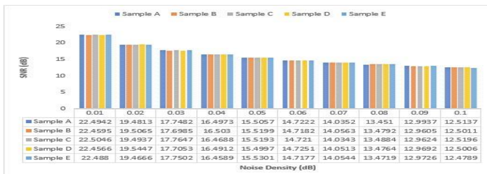
Fig. 7. SNR (dB) value versus Noise Density for Sample A, B, C, D, E
